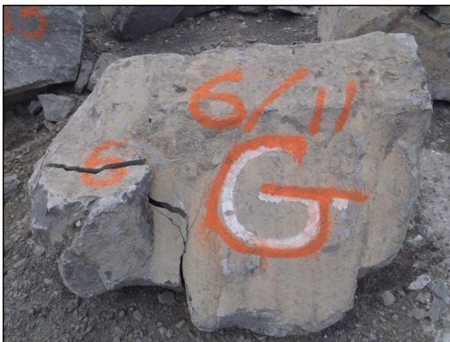
Figure 9. Fractured riprap stone in the site test
