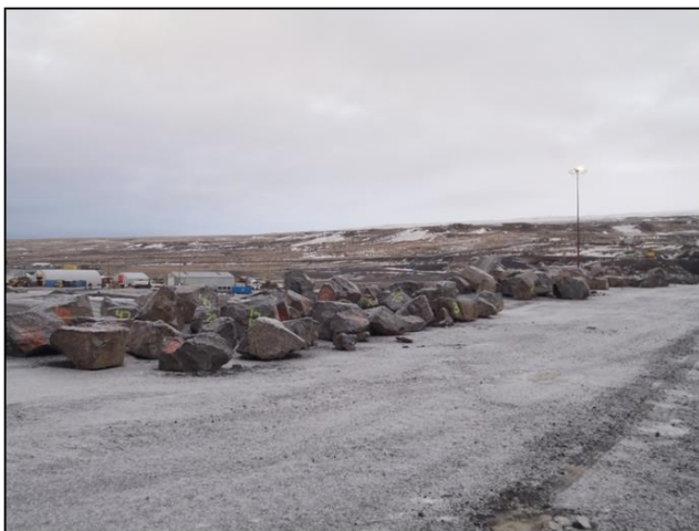
Figure 8. Site test of riprap stones
